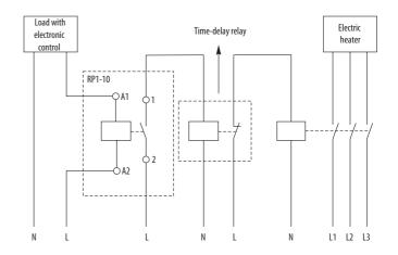
At priority switching of an appliance with electronic control the relay function is troubled (the relay is synchronized with the electronic control). For this reason it is recommended to connect a time-delay relay in the control contact circuit.
