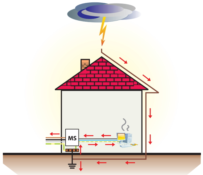
Stroke to the building Big installation threat
