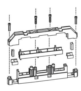
Methods of mounting SST-60/49-5 in the switchboard with two screws M6
